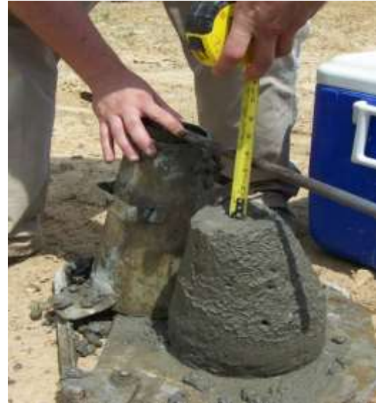
Fig.No-5.2.1 B) Slump Cone Test
