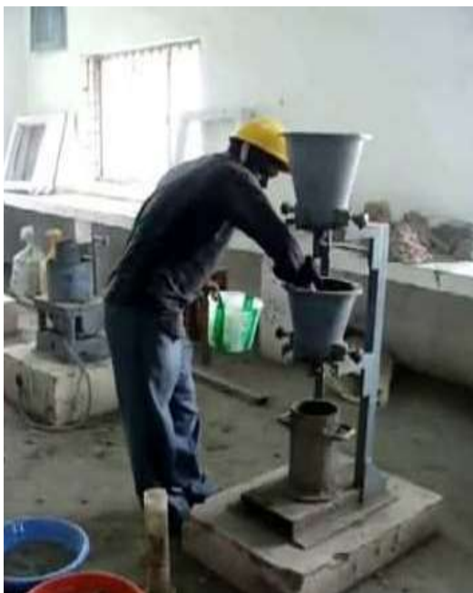
Fig.No-5.2.2 Compaction Factor test
